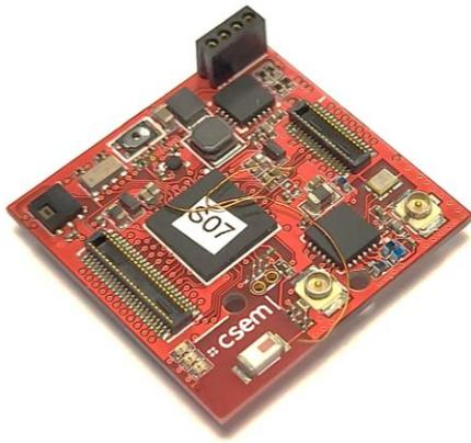
Fig. 2: The communication PCB (25 × 25 mm)
