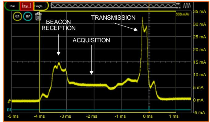
Fig. 20: Communication PCB power consumption during a beacon reception, acquisition and data transmission cycle. The sensor PCB current consumption is not included in this measurement.
