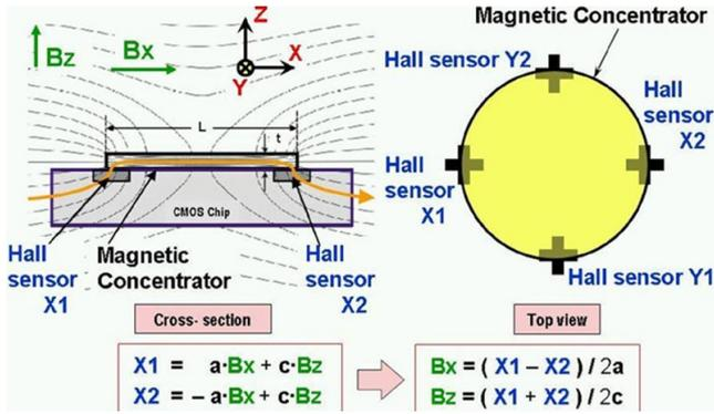
Fig. 6. Illustration of the 3-axis magnetic field sensor based on IMC-Hall technology (Courtesy of AKM, Japan.)
