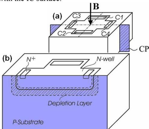
Fig. 1. Integrated planar Hall device in bulk CMOS technology. (a) Layout; CP denotes a crossing plane. (b) View with the cross-section along CP. Metallization and oxide layers are not shown.
