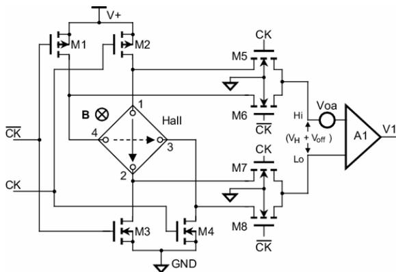
Fig. 3. A simple implementation of the Hall spinning-current biasing circuit. The whole system is shown in Fig. 4.
