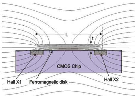
Fig. 5. IMC-Hall: Integrated combination of a planar magnetic flux concentrator and horizontal Hall devices.
