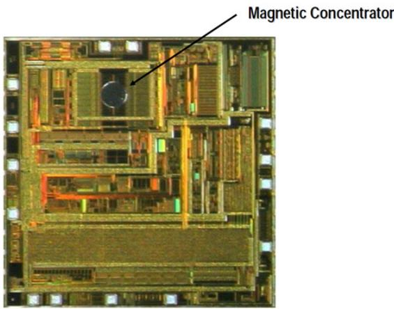
Fig. 7. Photograph of the 3-axis integrated compass chip based on the IMC-Hall technology, as illustrated in Fig. 6. This chip is applied as electronic compass in mobile phones.
