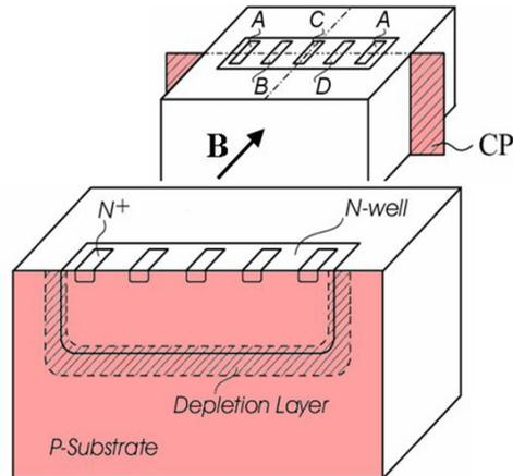
Fig. 2. Integrated vertical Hall device in bulk CMOS technology. (a) Layout; CP denotes a crossing plane. (b) View with the cross-section along CP. Metallization and oxide layers are not shown.
