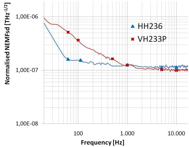
Fig. 8. Measured noise-equivalent magnetic field spectral density of the SENIS' Hall devices implemented in  $0.35\mu\text{m}$  CMOS technology, normalized to biasing power of  $1\text{mW}$ . HH236: horizontal Hall device ( $S_V = 0.038\text{T}^{-1}$ ,  $R = 3\text{k}\Omega$ ); VH233P: vertical Hall device ( $S_V = 0.043\text{T}^{-1}$ ,  $R = 1.9\text{k}\Omega$ ); Bias voltage (both):  $1\text{V}$ .
