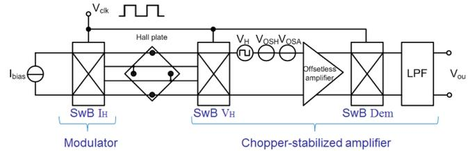
Fig. 4. Block diagram of the Hall spinning current biasing and signal conditioning system. Notation: SwB: Switching Box;  $I_H$ : Hall biasing current;  $V_H$ : Hall voltage; Dem: Demodulator.
